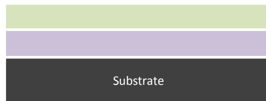
Figure 3.8. Condition for double layer w-type antireflection coating.
