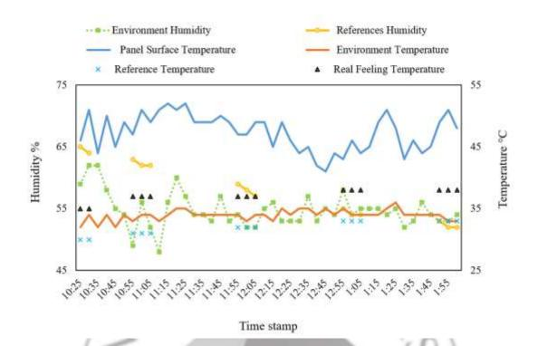
Figure 4.1-5: Difference temperature between solar panel and environment
