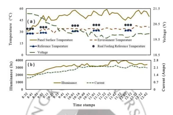
Figure 4.1-6: Comparison effect on solar panel output voltage
