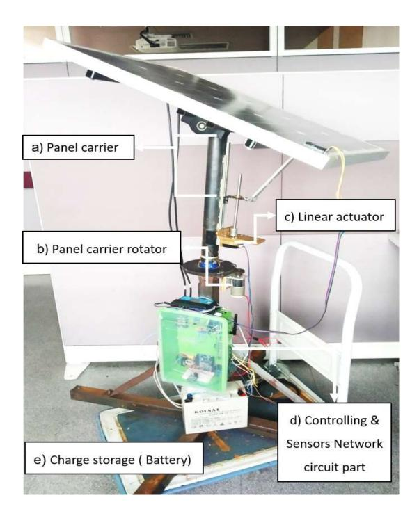
Figure 3.4-1: Structure of open loop tracking system
