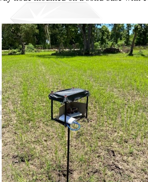
Figure 3.4: Receiver gateway node mounted on a solid base with cover protection.
